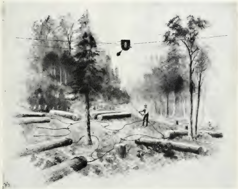
FIG. 52. HIGH LEAD OVERHEAD SKIDDING: THE BUNCHING LINE. [By courtesy of Messrs. Lidgerwood.]
